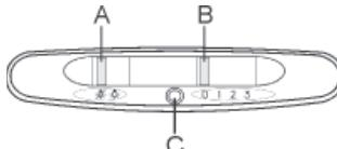
Switch A: LIGHT; position : light off; position : light on.
